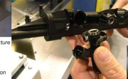
Assembling the injector into the fuel rail
