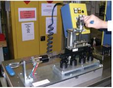
Testing the assembled fuel rail for leaks
