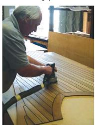
Construction of a Moody off-boat deck is a precision process, carried out by a mixture of the latest hightech machinery and highly skilled craftsmen. For standard production boats, the teak strips are produced by CNC machine following design by CAD and assembled into jigs that position the strips exactly, ensuring that the correct gaps are maintained, which will eventually be filled with caulking
