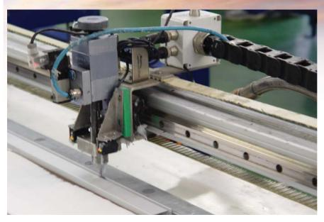
Automatically applying the silicone
