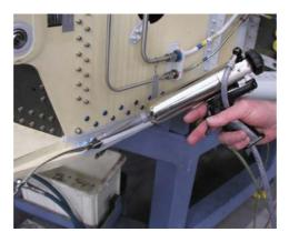
Applying mixed sealant from a cartridge gun
