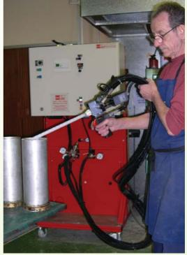
Dispensing the resin into moulds
