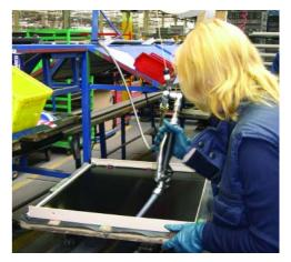
Merloni produces approximately 700 ceramic hobs every day, each one of which is sealed using this process. It is estimated that savings in material alone are in the region of £40,000 per year, simply from purchasing the silicone in bulk, resulting in an outstanding return on investment.
