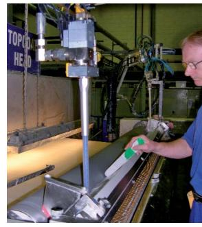
Mixing and dispensing the silicone coating onto the fabric web
