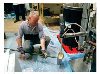
Filling the roller coater with mixed polyurethane
