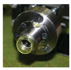
An end view of an applicator, clearly showing a metered shot of grease that would normally be injected into a bearing
