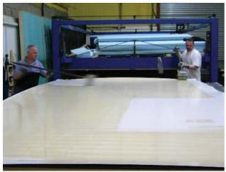
Laying the polyurethane onto a panel
