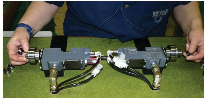
The operator offers up bearings to the twin DOPAG cartridge type metering valve
