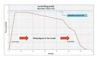
Diaphragm - Volumetric flow profile is defined by the mould filling time.
