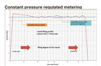
Constant pressure through volumetric flow.
