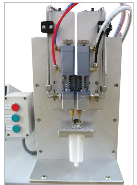
The syringe dispensing station showing twin DOPAG dispensing valves
