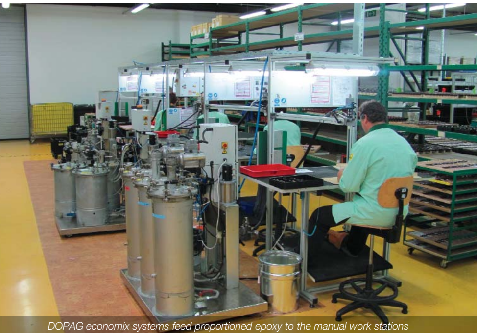
Dispensing the mixed epoxy into the electronic assembly
