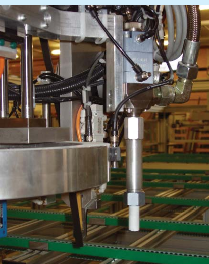
A DOPAG membrane dispensing valve and nozzle is mounted onto the robot ready for dispensing the sealant
