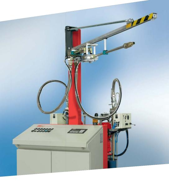
DOPAG Metering and Mixing System for pasty media TOOLING-MIX
