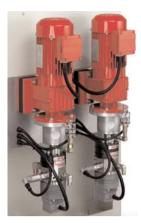
Material supply modules with pressure vessels are used to supply the material into the three phase asynchronous motor driven gear pumps where they are proportioned at the pre-selected ratio.
